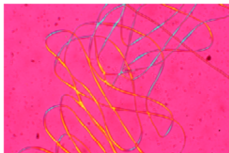
Figure 1: Polarizing optical microscope image of electrospun liquid crystal containing fiber viewed through cross polarizers and a retardation plate.
